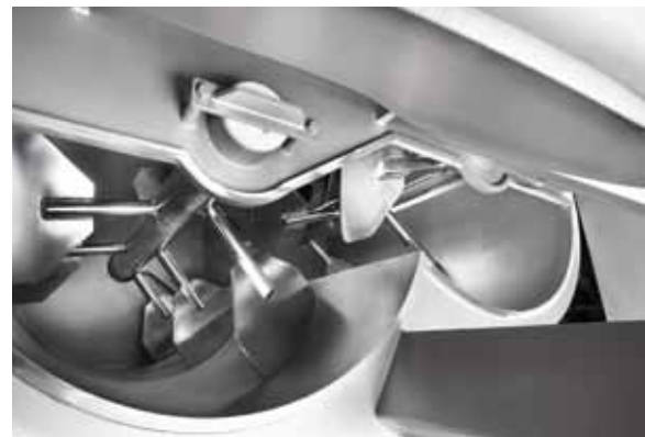
Discharge section of a TSMI
